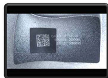
DPM Shield™ After Sandblasting Black Anodized Aluminum plate with direct part marking virtually destroyed by sand blasting except for area protected by DPM Shield™.
